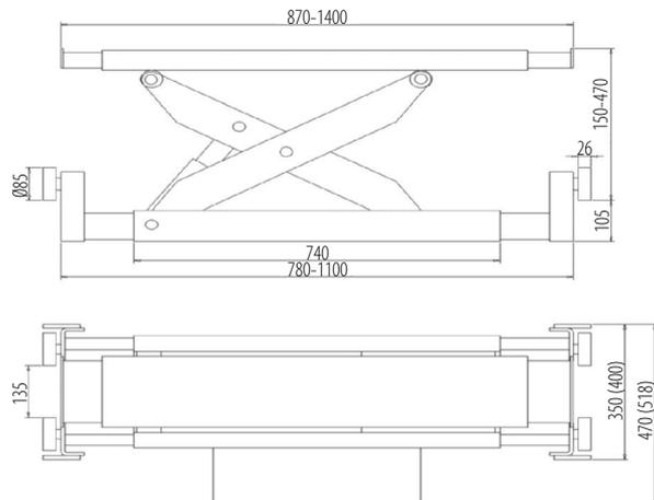
Electrohydraulic lift for geometry ♦ platforms with grooves for turntables and expansion plates ♦ mechanical height lock released pneumatically ♦ adjustable position of one platform ♦ perfectly secured hydraulic actuator ♦ galvanised ropes initially stretched ♦ rope wheels with large diameter ♦ lift lock while slackening or breaking ropes ♦ lift steering with safe voltage 24V ♦ safe device compatible with norm EN1493:2010.
